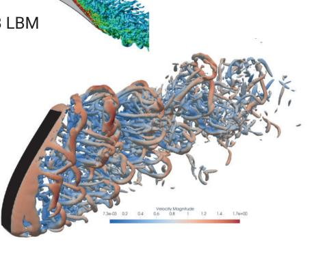
Visualization of the flow structures in the wake of a flexible plate
